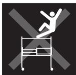
**DO NOT STAND OR ATTEMPT TO CLIMB THE PLATFORMS WHEN THEY ARE INSTALLED ON THE UPPER RUNG OF THE STRUCTURE**
